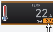
By turning the turn control to the left or right, adjust the set value (e.g. to 37.0 °C).
