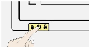
Press the main switch on the ControlCOCKPIT and disconnect the power plug. This disconnects the appliance from the power supply at all poles.
