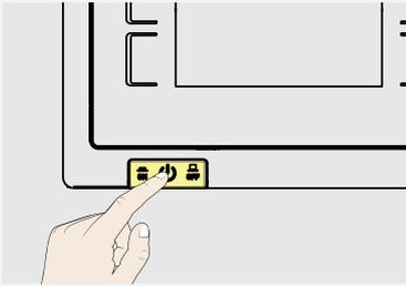
Press the main switch on the front of the appliance.
