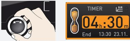
2. Turn the turn control until the desired duration is displayed – in this example 4 hours 30 minutes. The approximate end time is shown beneath, in a smaller font.
