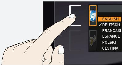
1. Activate the desired parameter (in this example the language). To do so, press the corresponding activation key on the left or right or the respective display. The activated display is enlarged.
