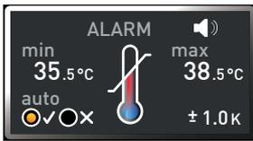
The monitoring temperature of the electronic temperature monitoring is measured via a separate PT100 temperature sensor in the chamber. Temperature monitoring settings are made via the ALARM display. The settings made apply to all operating modes.
