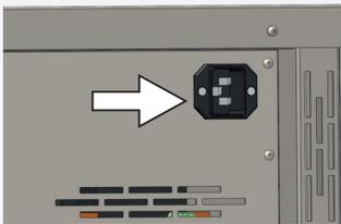
Observe the country-specific regulations when making connections (e.g. DIN VDE 0100 with earth leakage circuit breaker, in Germany). Observe the connection and power ratings (see name plate and the "Technical Data" chapters 2.7 and 2.8). Make sure to establish a safe PE conductor connection.
