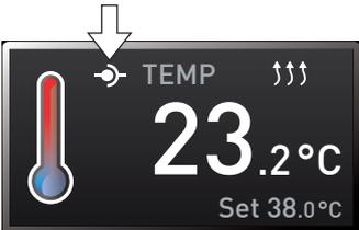
If the appliance is in remote control mode, the
