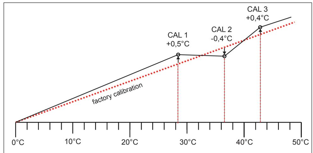
Example: Temperature deviation at 30°C is to be corrected
