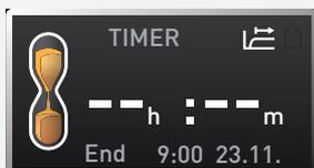
To- the timer, open the timer display by pressing the activation key again and then turning the turn control to reduce the timer setting until --:-- is displayed. Press the confirmation key to confirm.
