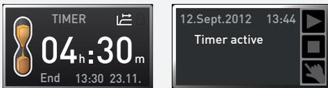
The display now shows the remaining time in a large font and the approximate end time in a smaller font beneath. The status display shows Timer active.
