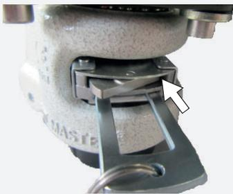
The direction of movement (up/down) can be adjusted using the rocker above the ratchet lever:
