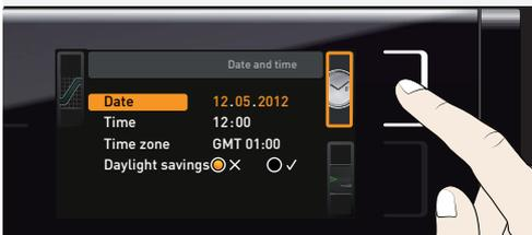
1. Activate the time setting. To do so, press the activation key on the right side of the TIME display. The display is enlarged and the first adjustment option (Date) automatically highlighted.
