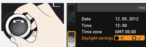
7. Set daylight savings to off (X) or on (O) with the turn control – in this case on (O). Save the setting by pressing the confirmation key.
