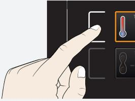
If you want to cancel the setting procedure, press the activation key on the left or right of the display that you want to exit. The appliance restores the former values. Only the settings that you have confirmed by pressing the confirmation key before cancelling the setting procedure are accepted.
