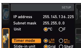
Here, you can choose whether the digital backwards counter with target time setting (timer, chapter 5.3.2) should run setpoint-dependent or not – this determines whether the timer should not start until a tolerance band of  $\pm 3$  K around the set temperature is reached ( B ) or whether it should start right after activation ( A ).
