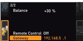
The setup entry gateway is used to connect two networks with different protocols. The gateway is set the same way as the IP address (chapter 7.3.2).
