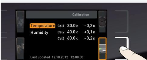
1. Press the activation key to the right of the CALIB display. The display is enlarged and the temperature adjustment option is automatically selected.
