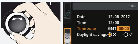
4. Use the turn control to adjust the time zone on the appliance location,
