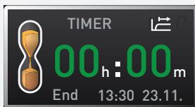
Once the timer has finished, the display shows 00h:00m. All functions (heating etc.) are switched off. In addition, an acoustic alarm sounds, which can be turned off by pressing the confirmation key.
