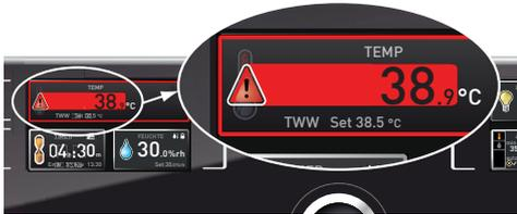
The monitoring temperature of the electronic temperature monitoring is measured via a separate PT100 temperature sensor in the chamber. Temperature monitoring settings are made via the ALARM display. The settings made apply to all operating modes.
