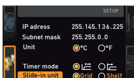
Here, you have to select the type of slide-in unit (steel grid or shelf) used. The selection Shelf enables you to adjust the control function to the different air flow characteristics in the interior when using optional sliding shelves instead of the steel grids that are provided as standard.
