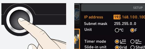
2. Accept the selection by pressing the confirmation key. The first three digits of the IP address are automatically selected.
