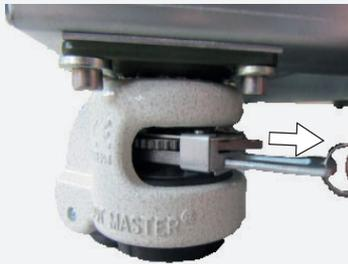
1. To unlock the adjustment mechanism, pull out the ratchet lever on the ring
