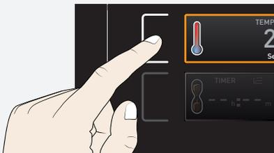
Activate the desired parameter (e.g. temperature). To do so, press the corresponding activation key on the left or right or the respective display. The activated display is lined in colour, the other displays are dimmed. The set value is highlighted in colour.
