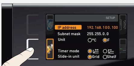
1. Activate the SETUP display. The entry IP address is automatically highlighted.
