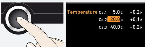
2. Press the confirmation key repeatedly, until the calibration temperature Cal2 is selected.
