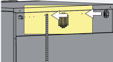
1. Tighten the tilt protection onto the back of the appliance as illustrated.
