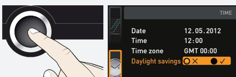
6. Accept the selection by pressing the confirmation key. The adjustment options are highlighted.
