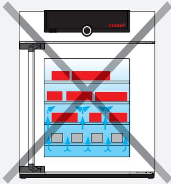
The chamber must not be loaded too tightly, so that proper air circulation in the interior is guaranteed.
