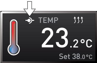
If the appliance is in remote control mode, the
