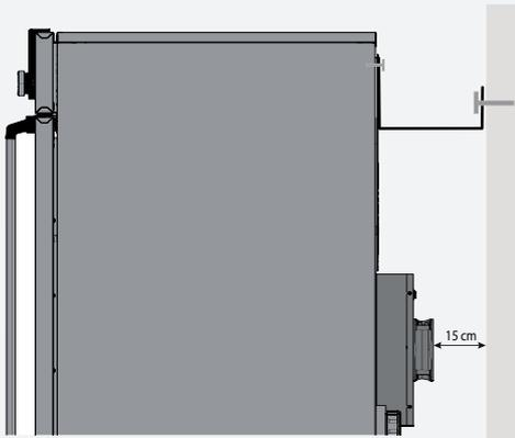
2. Bend the tilt protection upwards by 90° in the desired distance to the wall (observe the minimum distance to the wall).
