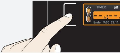
1. Press the activation key to the left of the timer display. The timer display is activated.
